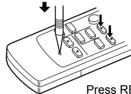
Press RESET button gently using a thin instrument.
