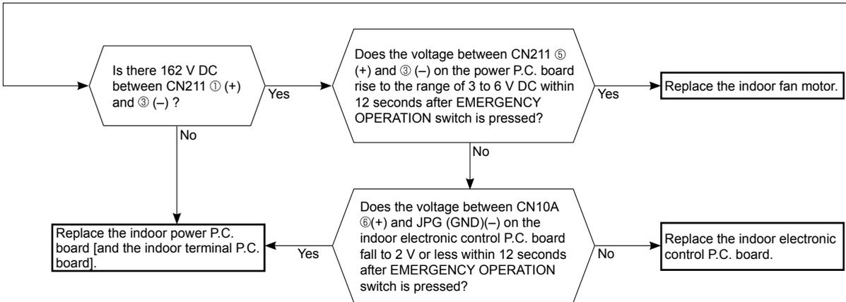
The indoor fan motor error has occurred, and the indoor fan repeats "12-second ON and 30-second OFF" 3 times, and then stops.
