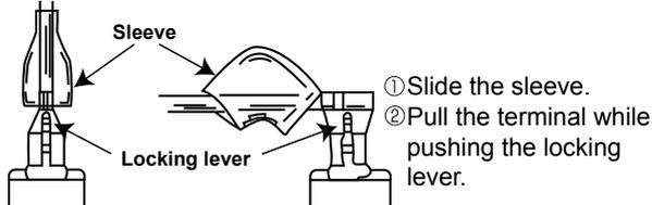
(2) The terminal with this connector shown below has the locking mechanism.
