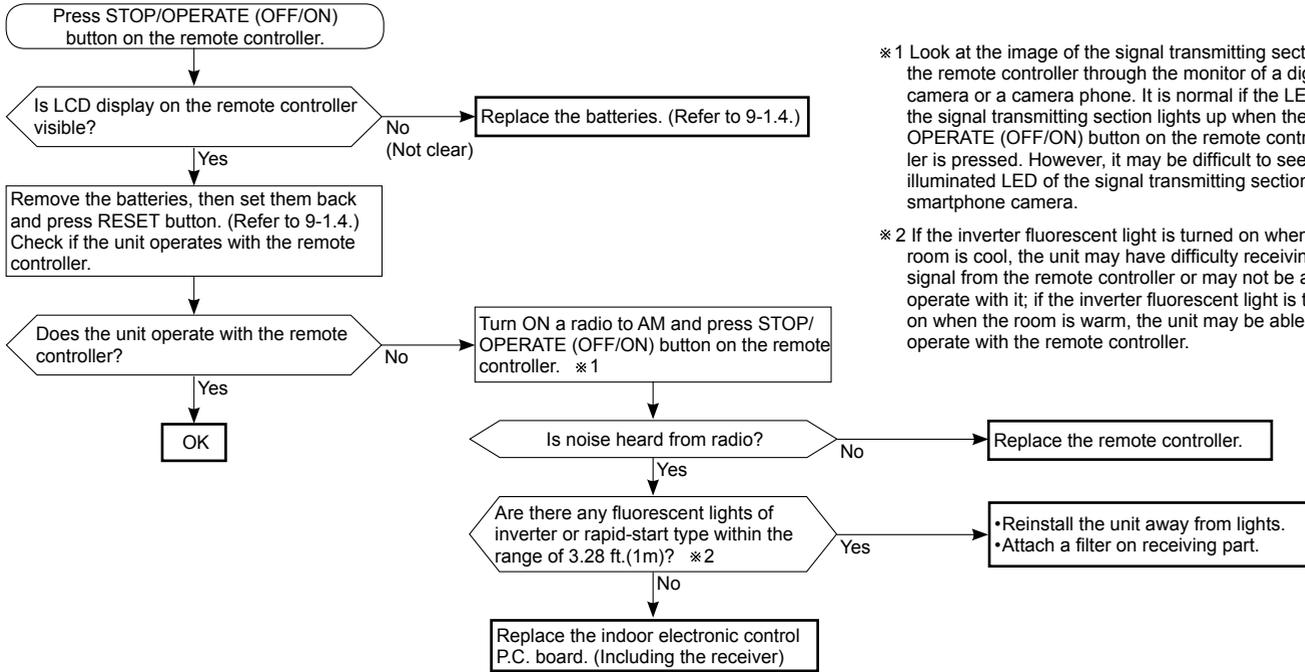
※1 Look at the image of the signal transmitting section of the remote controller through the monitor of a digital camera or a camera phone. It is normal if the LED of the signal transmitting section lights up when the STOP/OPERATE (OFF/ON) button on the remote controller is pressed. However, it may be difficult to see the illuminated LED of the signal transmitting section with a smartphone camera.
