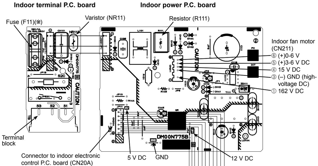
※ Please replace the fuse after removing the indoor terminal P.C. board from the electrical box.
